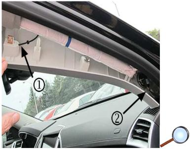
1. Starting on the left or right side, remove the windshield garnish molding from the A-pillar by pulling gently from the top to disengage the attachment clip. Detach the rubber stop (1) on the tether clip from the molding and disconnect the speaker wiring harness (2).
