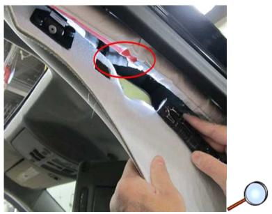
4. Pull the front corner of the headliner downward to access the drain hose and sunroof drain spigot connection, circled above.
