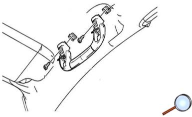
3. Remove the front assist handle. Refer to Front Assist Handle Replacement in SI.
